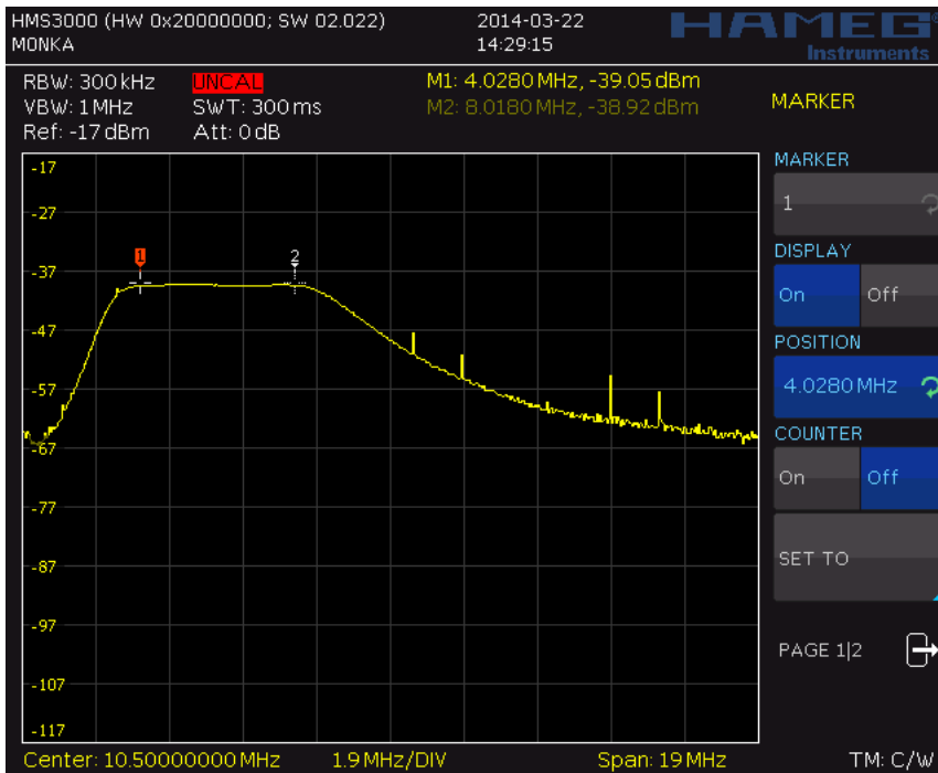
Fig3: Filter response for 40m band
