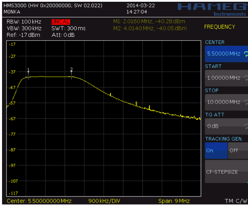
Fig2: Filter response for 80m band
